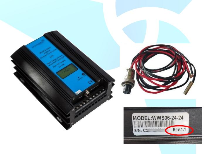
**NOTE:** To identify the revision, check the serial number label placed on the left side of the charge controller. If <u>no revision is written on the label</u>, you can assume that is revision 0.
